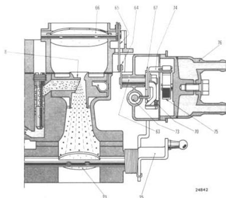
ADF and ADL Carburetors have a water activated choke mechanism (76). Hot water tensions a spring that activates a lever (64/65) and holds the choke plate (66) open. It is an effective and simple system.
